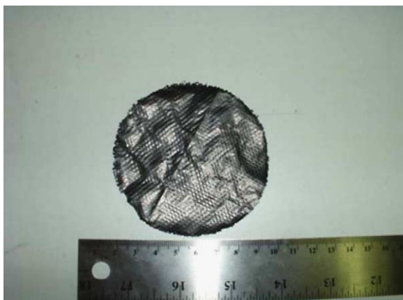
Fig. 1. Ninety millimeter diameter SWNT buckypaper.
